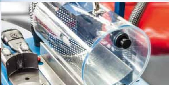
For these problematical cases, Fuchs Umwelttechnik developed the combination of pre-separator system and downstream filter system. Large parts which were accidentally or believed lost are now caught already by the pre-separation module and are visible all the time thanks to its transparency. Finer material such as dusts or gases flow on unobstructed into the downstream filter system.
